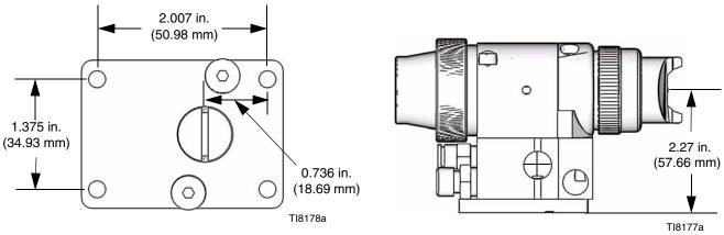
Fig. 30: Mounting Hole Layouts
